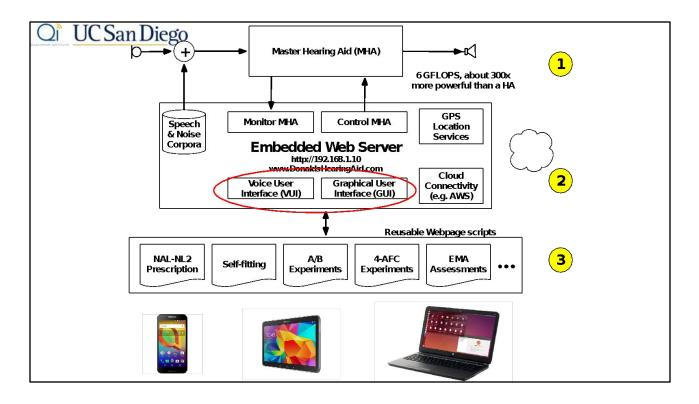
Graphical interfaces within the web pages served by the embedded web server access a straightforward API to obtain and send the hearing aid parameters. This gives the researcher the option to create a simple web page in plain HTML for rapid prototyping, or a feature-rich web page with JavaScript for more custom interfaces.
