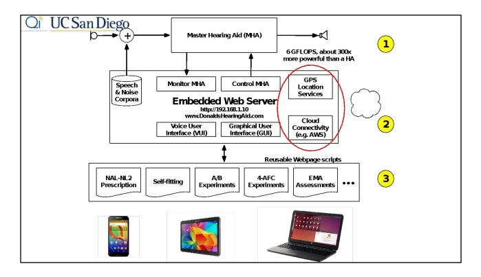
For the embedded version of the platform, since it is based on a chipset from commercial smartphones, we have GPS for location based capabilities. With this we can change the state of the hearing aid based on location, and assess the state of the user using Ecological Momentary Assessments.
